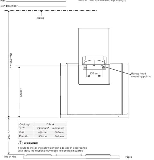
1. Using a spirit level mark a vertical centre line on the wall where the cooker hood is to be positioned, and a horizontal line at the cooker hood base position (refer diagram below).
