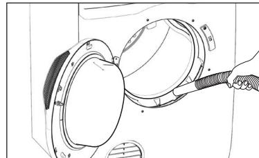
① If necessary remove fluff from the filter socket and gasket. You can use a vacuum cleaner.
