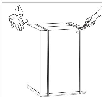
2. Remove the carton box. Remove the polystyrene packaging materials. Remove the plastic bag which cover the machine.
