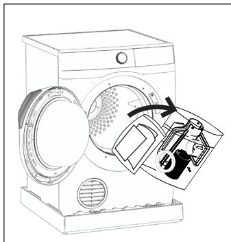
4. Put one of the polystyrene packaging elements on the floor behind the appliance. Carefully put down the appliance with the rear side on it.
