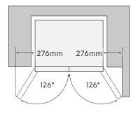
When positioned in a corner area, spacing of at least 276mm on the right hinge side and 276mm on the left hinge side will allow the doors to open enough to enable the removal of bins and shelves.
