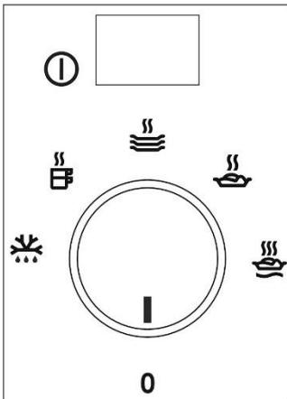
The control panel has a selector and an on/off switch. The control panel is only visible when the drawer is open.
